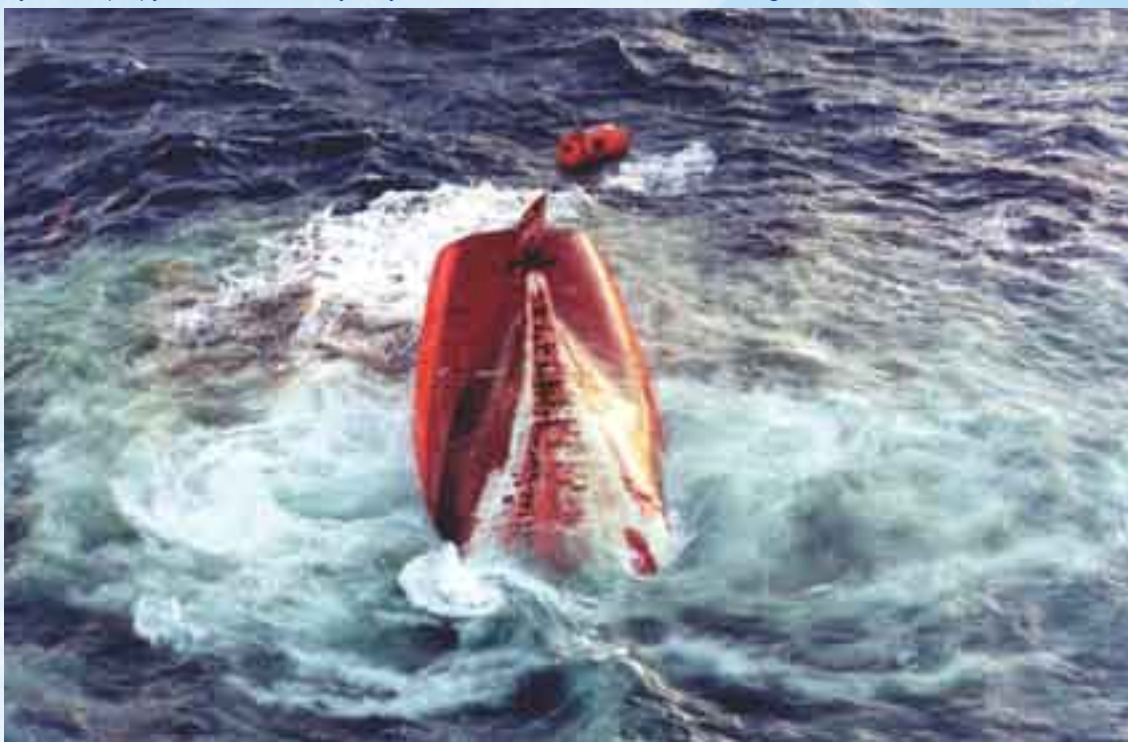
The 2001 sinking of the levoli Sun in the Channel Islands, UK, after taking on water in heavy weather. The vessel was carrying styrene, isopropyl alcohol, and methyl ethyl ketone as well as intermediate fuel oil, gas oil, and lubricants.
